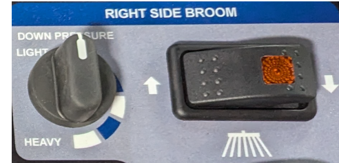
Fig. 40: Side Broom Down Pressure Knob
