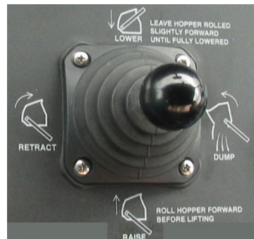
Fig. 29: Hopper Dump Lever
