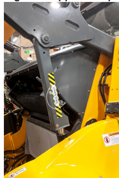
Fig. 33: Hopper Safety Supports
