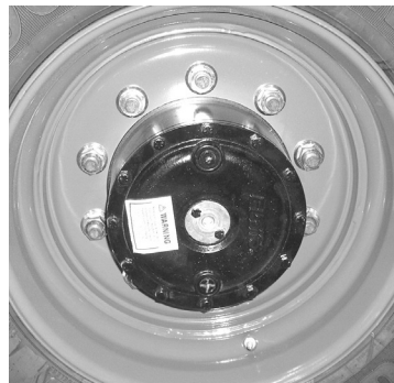
Fig. 70: Drive Hub—Drain Position
