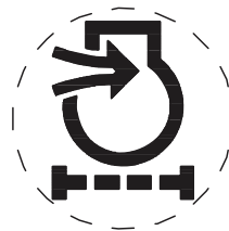
Fig. 48: Air Filter Restriction Indicator
